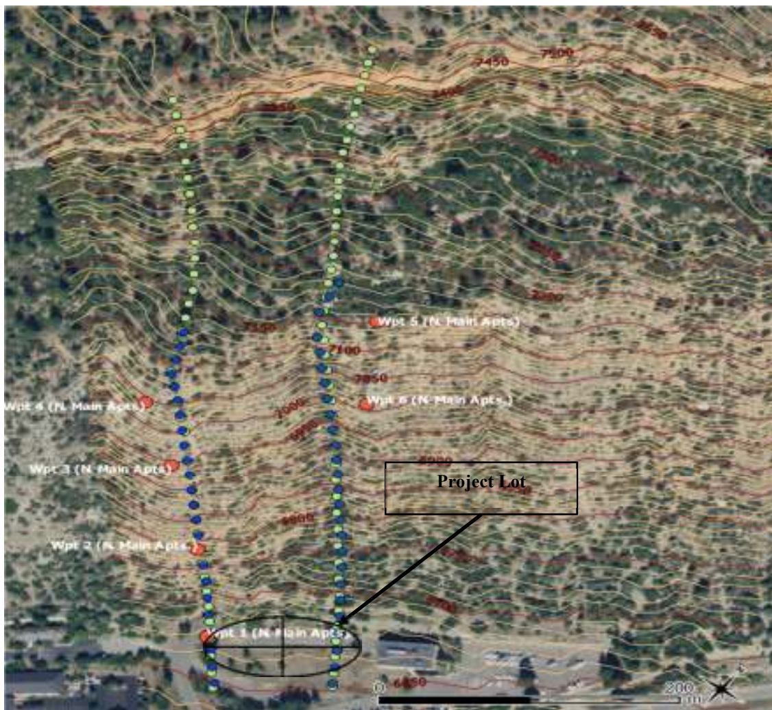
Figure 4: Vicinity Map and Aerial Photo showing topography (10 foot contour interval), lot location, rockfall paths analyzed in CRSP (blue dots show below upper bench path, green dots show full path), and handheld GPS waypoints (orange dots) from field reconnaissance
